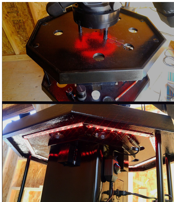
Top and Bottom Bottom Pier Shelf Illumination (Note Dimmer in Bottom Photo)
